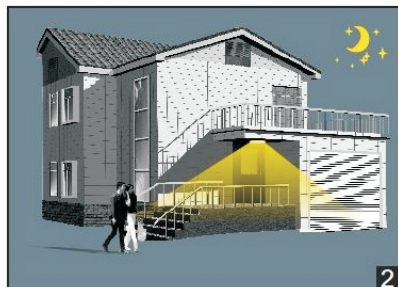
With insufficient daylight,even when motion detected.light ON.
